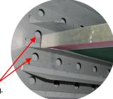
**Dynamic Air Flow** above and below the screens ensures consistent & even drying.
