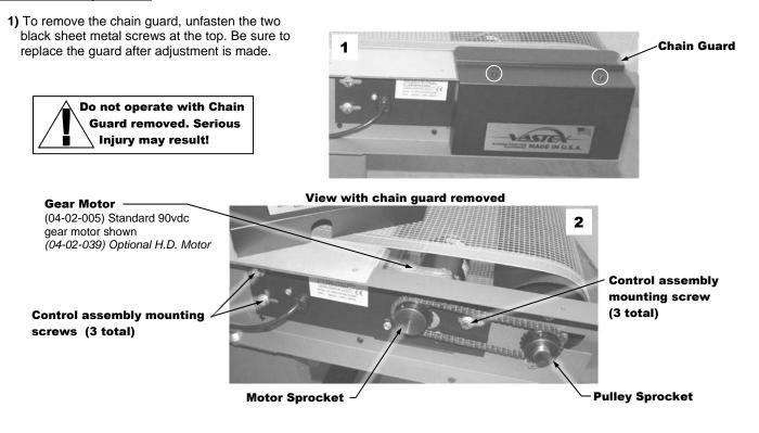
2) To adjust the drive chain you will need to loosen the three Control assembly mounting screws. The Drive plate is slotted to allow the entire assembly to slide left or right to loosen or tighten the chain. Adjust the chain so there is approximately 1/4" of vertical movement in the chain.
