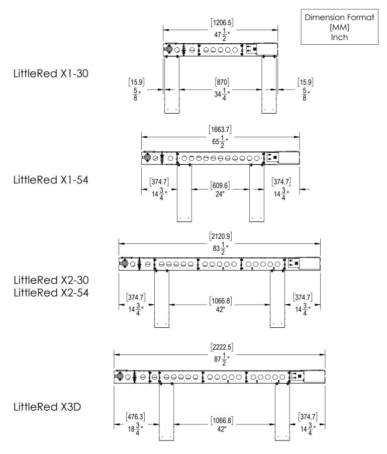
XX-30= 30"(762mm) Belt, 35.8"(909mm) Conveyor Width XX-54= 54"(1372mm) Belt, 59.8"(1519mm) Conveyor Width
