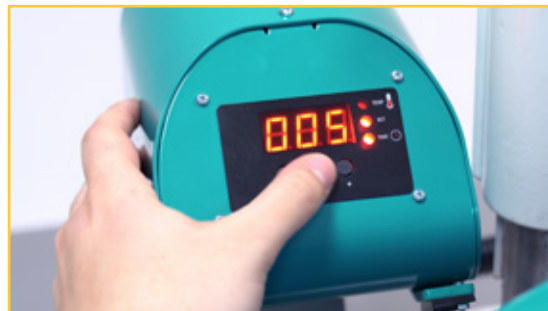
Press MODE twice to set the TIME. While SET and TIME are illuminated, press (+) and (-) buttons to adjust the TIME.
