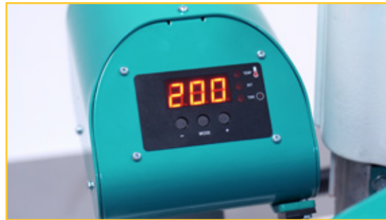
While no LEDs are illuminated, the controller displays the current heater temperature. Press the MODE button to set the TEMPERATURE and TIME.
