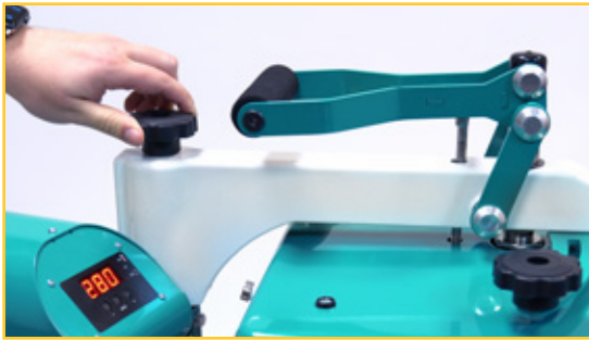
With the print handle in the raised position, rotate the knob to adjust PRESSURE.
